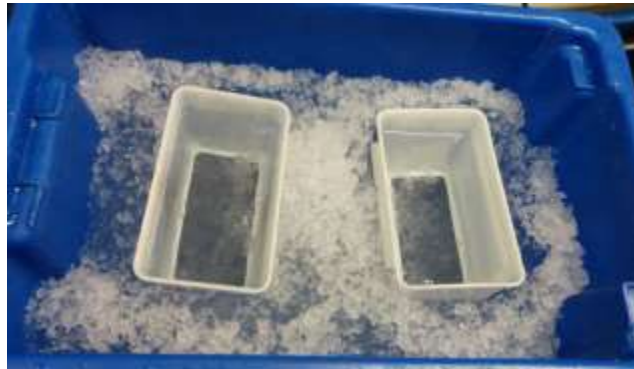
Figure 4- Strainers located in Ice slurry
