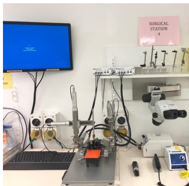
A. B. Figure. Example set ups for stereotaxic rigs. A) Manual set up and B) computerised stereotaxic rig
