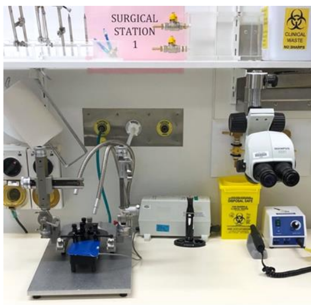
A. B. Figure. Example set ups for stereotaxic rigs. A) Manual set up and B) computerised stereotaxic rig
