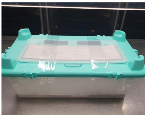
Figure 3 Placement of tape at two locations if taping closed (UQBR 2020).
