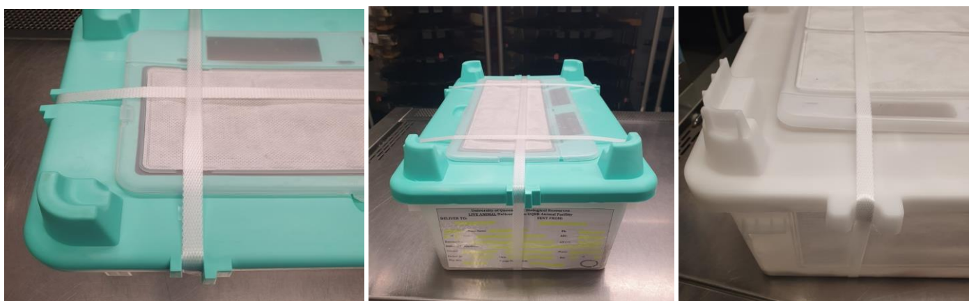
Figure 5. Placement of strapping if using automatic strapping machine.
