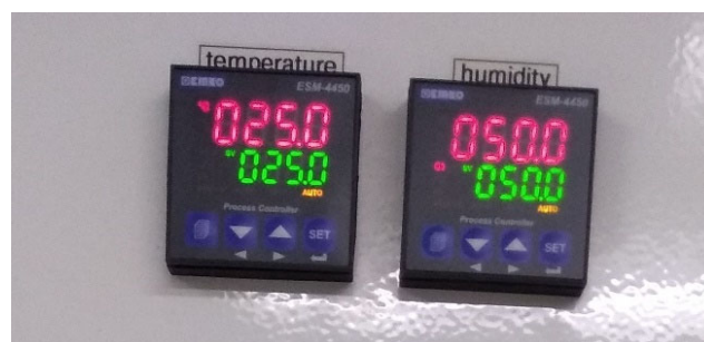
Figure 3: Manual light control (left), and digital set (green) and actual (red) temperature and humidity readings on chambers.
