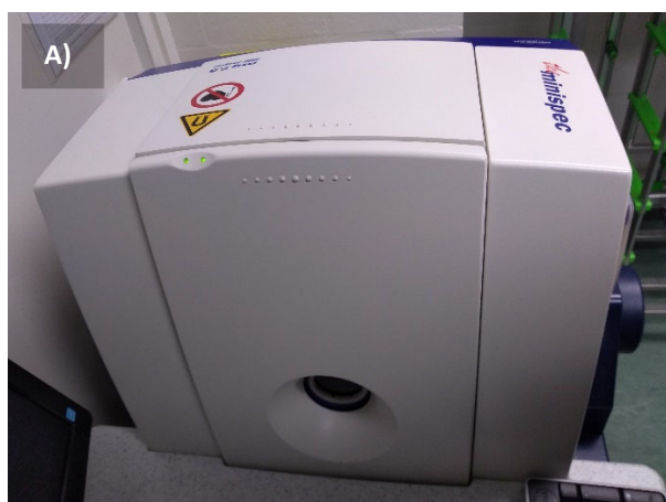
Figure 1A) NMR Minispec unit, by Bruker, and B) Rodent restraint tubes.
