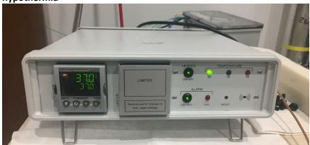
3. Fill the warm water circulation unit with distilled water. Set the water circulation at 45°C. The water temperature is set higher than physiological temperature to compensate for heat loss when the water flows through a long tubing, the animal bed and foam surfaces.
