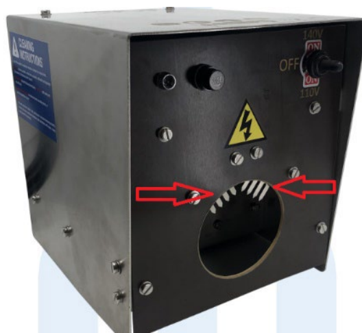
Figure 6 - Electric poultry stunner, electrode probes indicated by red arrows.
